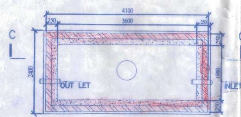
PLAN DETAIL OF S.U.G. TANK SCALE 1:50
